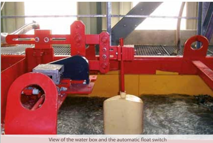
View of the water box and the automatic float switch
